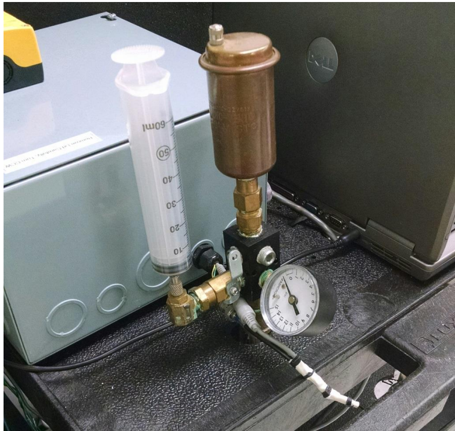
Figure III.3 – Pressure gauge for quickly monitoring the flow rate of the recirculation pump. The dissolved oxygen sample port is also visible in this picture, with the syringe body attached to the fitting. A small valve (shown in the off position) leads to this port.
