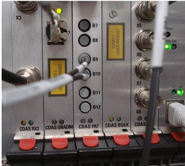
Figure III.5 – CDAS box for Philips 3T MRI systems. The fiber optic cables that carry the timing pulse (from the RS-232 serial converter) plug into the holes marked B9 and B10.
