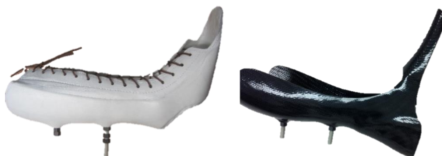
Figure 2.3. Hindfoot (white) and forefoot (black) ankle-foot orthosis. The bolts on posterior surface are for mounting to the HyPSTR loading frame.
